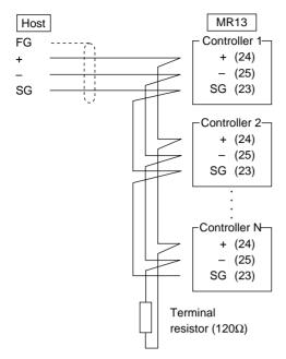
Note 1: In the case of RS-485, provide it with a terminal resistor of about 1/2W,  $120\Omega$  across terminals 24 and 25 if necessary.
